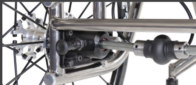
Piranha with single arm drive showing the removable drive axle
