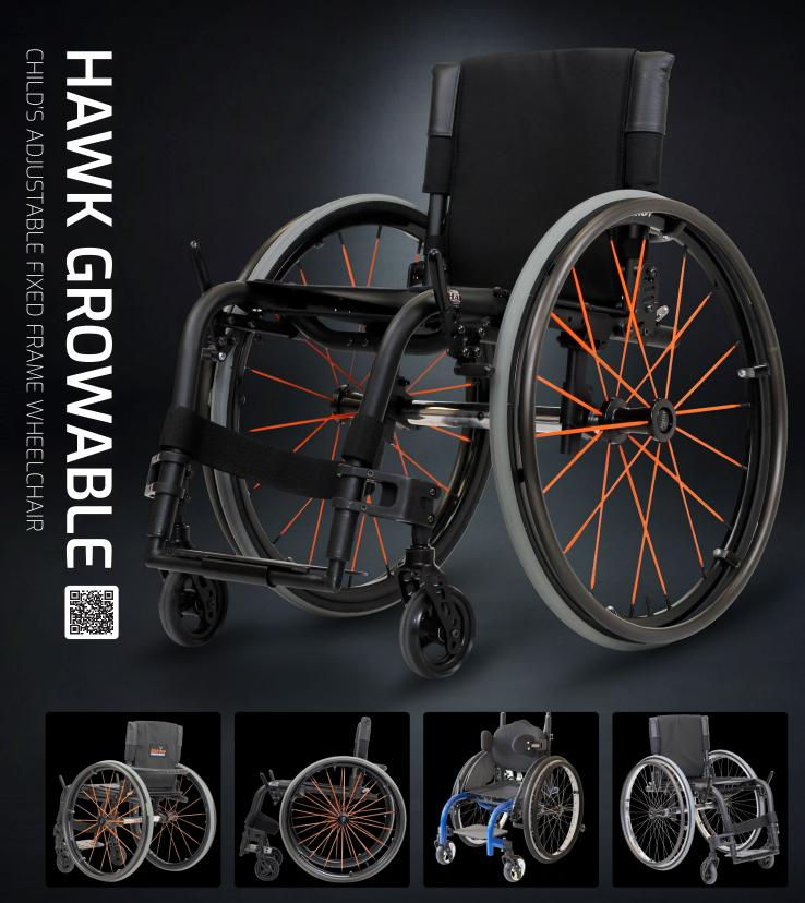
The Melrose Hawk Grow-able sits alongside its big brother as our main lightweight adjustable position wheelchair. Being able to grow in width and length allows for a longer period before having to move to a larger ride.
