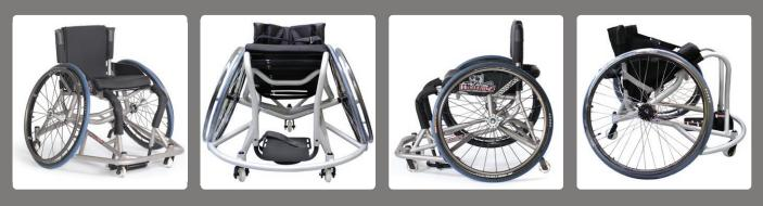
The Melrose Wolverine comes standard in lightweight aluminium, but can also be built in titanium for a super light super responsive frame.
